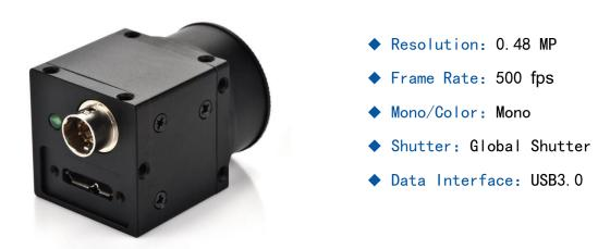
U3SMT50GM is a brand-new USB3.0 industrial camera launched by our company. The transmission speed of USB3.0 series is greatly improved compared with USB2.0 and GigE camera. The transmission bandwidth of 5Gbps can still have higher frame rate and faster transmission speed under high pixels with high-speed sensor. The size is only 29mm x 29mm x 29mm. The USB3.0 interface has a locking seat. It is plug and play without power supply, and can be flexibly installed in different structures.
