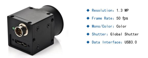
U3SMT131GC is a brand-new USB3.0 industrial camera launched by our company. The transmission speed of USB3.0 series is greatly improved compared with USB2.0 and GigE camera. The transmission bandwidth of 5Gbps can still have higher frame rate and faster transmission speed under high pixels with high-speed sensor. The size is only 29mm x 29mm x 29mm. The USB3.0 interface has a locking seat. It is plug and play without power supply, and can be flexibly installed in different structures.
