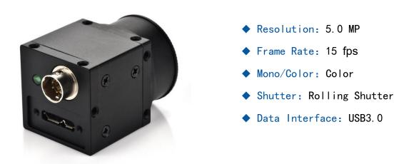
U3SMT500C is a brand-new USB3.0 industrial camera launched by our company. The transmission speed of USB3.0 series is greatly improved compared with USB2.0 and GigE camera. The transmission bandwidth of 5Gbps can still have higher frame rate and faster transmission speed under high pixels with high-speed sensor. The size is only 29mm x 29mm x 29mm. The USB3.0 interface has a locking seat. It is plug and play without power supply, and can be flexibly installed in different structures.
