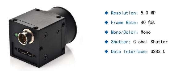
U3SMT501GM is a brand-new USB3.0 industrial camera launched by our company. The transmission speed of USB3.0 series is greatly improved compared with USB2.0 and GigE camera. The transmission bandwidth of 5Gbps can still have higher frame rate and faster transmission speed under high pixels with high-speed sensor. The size is only 29mm x 29mm x 29mm. The USB3.0 interface has a locking seat. It is plug and play without power supply, and can be flexibly installed in different structures.
