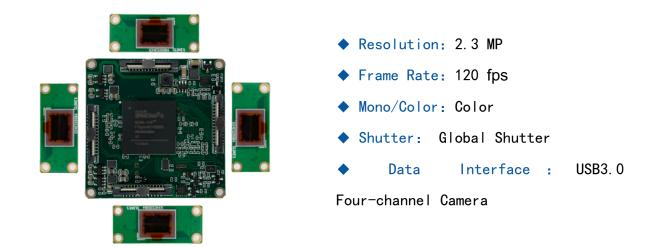
U3BMT200GC-4C is a new generation product that our engineers have fully optimized on the basis of the structure of the third generation four-channel product series, which greatly reduces the difficulty of process assembly and enhances the compatibility of the product. At the same time, the software functions have also been optimized to allow more camera functions to be implemented in the software code, reducing the use of logic resources; reducing power consumption and increasing compatibility.
